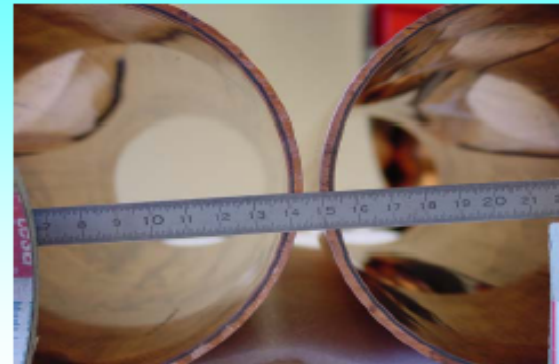
Hot roll bonded Cu-Nb-Cu tube produced at Nippon Steel Co.
