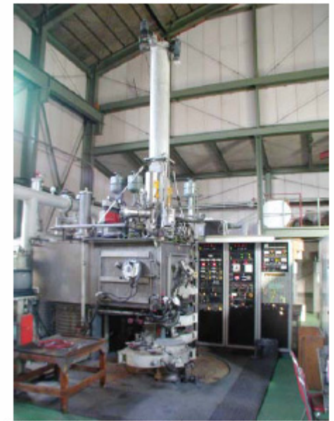
Electron beam melting furnace in Tokyo Denkai
